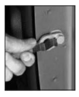
Release the retaining cable clip by lifting the cable so it is level with the ground and then push the cable clip toward the vehicle.
